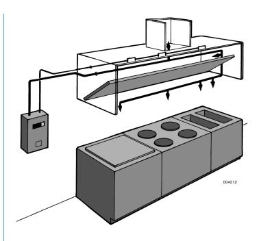
The system is capable of automatic detection and actuation as well as remote manual actuation. Additional equipment is available for building fire alarm panel connections, electrical shutdown and/or interface, and mechanical or electrical gas line shut-off applications.
